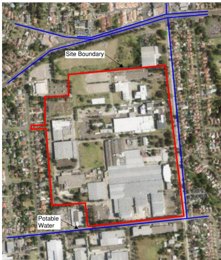
Figure 4 – Location of Potable Mains
